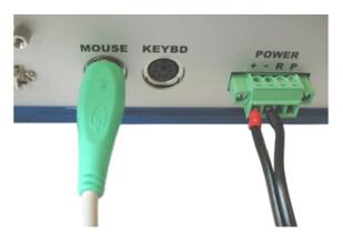
**2** Use a keyboard with a PS/2 connector and attach it to the back panel of your xPC TargetBox.
