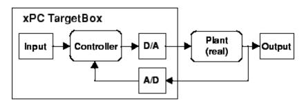
• Hardware-in-the-loop simulation — Test a real controller connected to a simulated plant running in real time on an xPC TargetBox.
