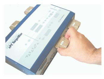
**2** Press the two latches on the sides of each dongle at the same time and remove the dongle from the connector.
