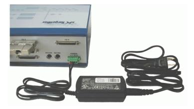
You are now ready to start the xPC TargetBox for self-testing. Because the xPC TargetBox does not have a power switch, the system starts to operate as soon as you plug the AC power cord into a wall outlet.
