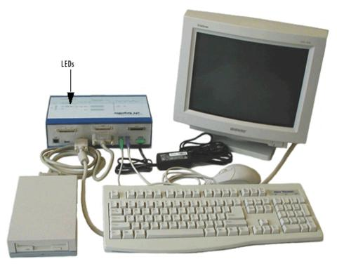
**4** After the BIOS loads (time varies with xPC TargetBox model), the floppy disk drive is accessed (verify by observing the green LED on the front of the external floppy disk drive and listening for an audible sound from the drive).
